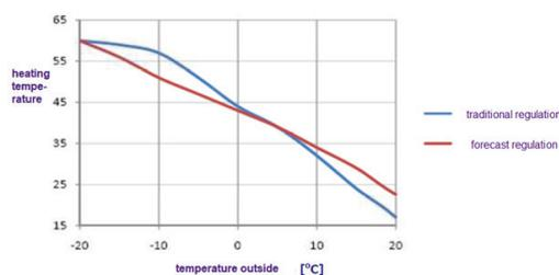
Fig. 1. Comparison of traditional and forecast adjustment [6]
