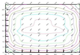
Fig. 5. Results of the simulation of the light intensity from light pipes in a sports hall [7]
